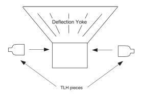
HTIL correction can be performed by adding a TLH correction assembly to the Deflection yoke.
